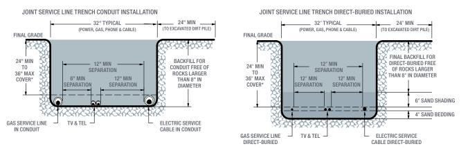
\*Check with local permitting agency for depth of cover requirements for any PSE facility installed in public right-of-way. 36" cover may be required over PSE facilities.
